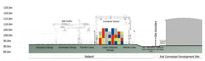
SECTION D - Direct Rail Connection with Side Platform Loading
