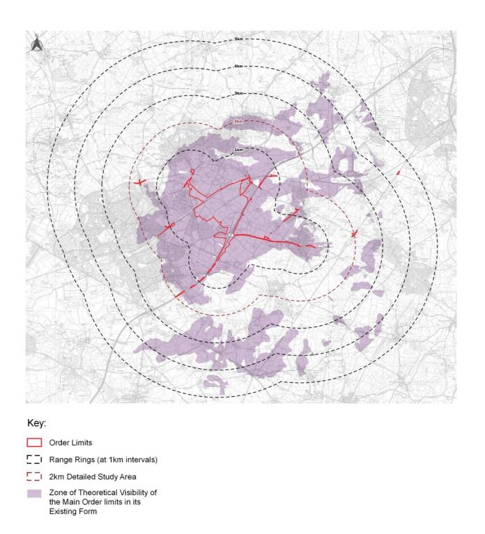
Fig 25. Zone of Theoretical Visibility of the Main Order Limits in its Current Form (Document Reference 6.3.11.7)
