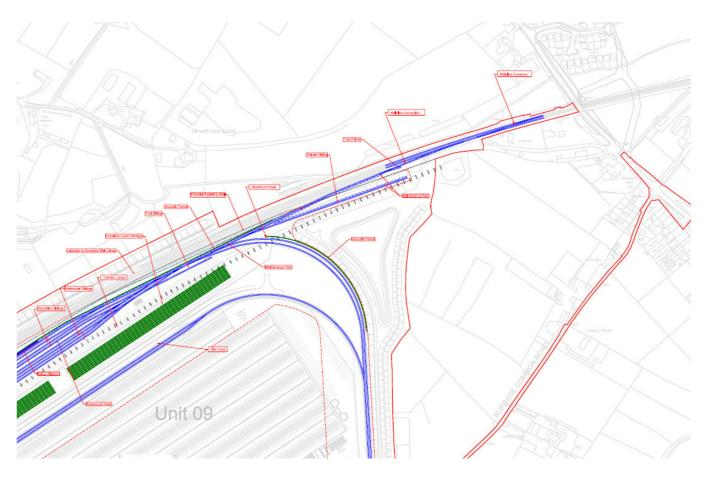
Fig 58. Eastern Arrangement of Main Reception sidings, intermodal sidings and container storage. Document Reference 2.25
