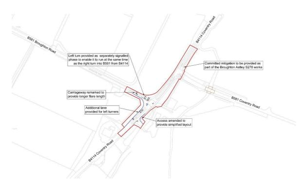
Fig 52. Proposed Works to Coventry Road / Broughton Road junction east of Stoney Stanton (Document Reference 6.3.3.3)
