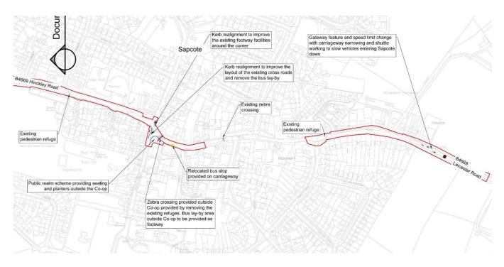
Fig 50. Proposed Works to the Hinckley Road / Leicester Road, Sapcote (Document Reference 6.3.3.3)
