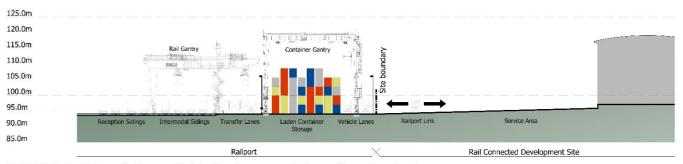
SECTION A - Direct & Secure Vehicular Access to Railport from Service Area
