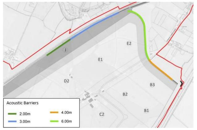
Fig. 61 Proposed Noise Barriers to north west of Railport and to the north east of head shunt (Document Reference 6.3.10.10)
